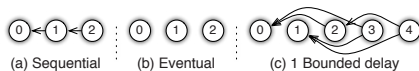
Figure 6: Directed acyclic graphs for different consistency models. The size of the DAG increases with the delay.
