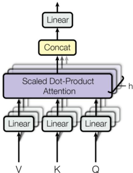
Figure: The single and multi-head attention layers of Vaswani et al. 2017.
