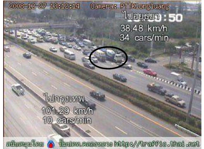
Fig. 2. Disruption precursor caused by a truck that blocked a lane.
