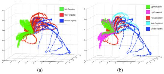
Figure 3. Clustering results of large-scale traffic dynamics (a) The number of clusters is 3. (b) The number of clusters is 5.
