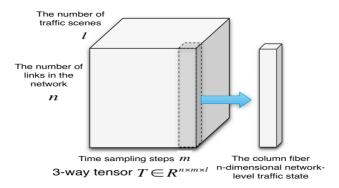
Figure 1. Structure of the traffic data 3-way tensor
