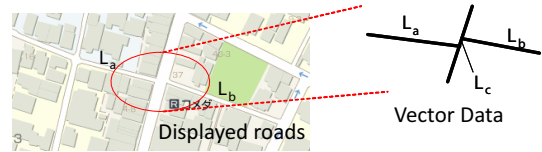
Figure 11: Intersection having slight misalignment.
