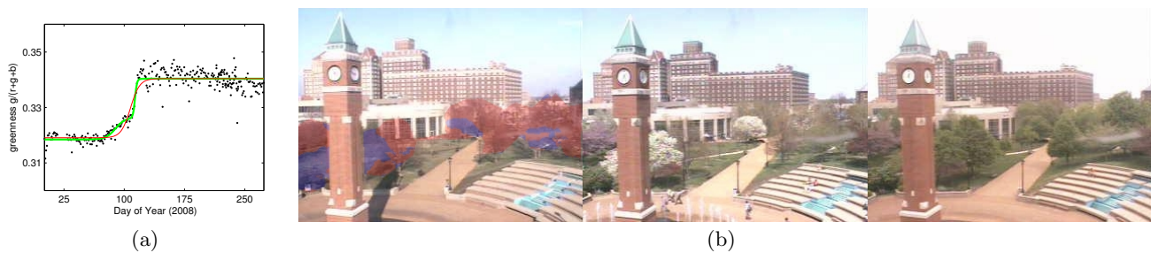
Figure 9: Using webcam images for phenological monitoring has advantages in operating at a much finer spatial and temporal resolution than satellite imagery. Here we show that the higher spatial resolution enables distinguishing between trees with different spring leaf growth rates. (a) The value of the greenness signal (black dots) for a camera viewing a clock-tower in a plaza. The thin (red) curve is the value of a single-sigmoid model fit to the data. The thick (green) curve is the value of a mixture-of-sigmoids model fit to the data. (b) A montage of images captured by the camera. The first image (left) has a color overlay that corresponds to which component of the mixture-of-sigmoids model best fits the time-series of the underlying pixel. The other images provide evidence that the segmentation is meaningful (the purple regions grow leaves earlier than the red regions).
