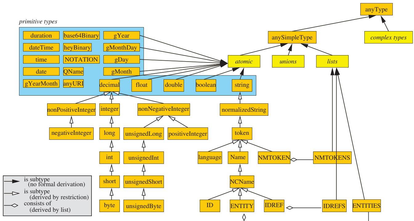
Figure 18: XML Schema built-in datatypes.
