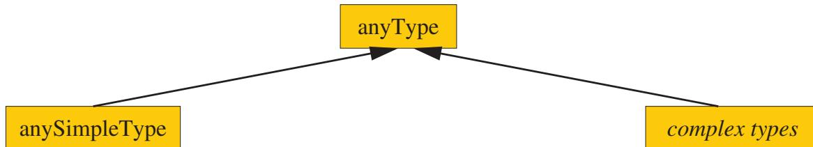
Figure 17: XML Schema Type hierarchy (top-level).
