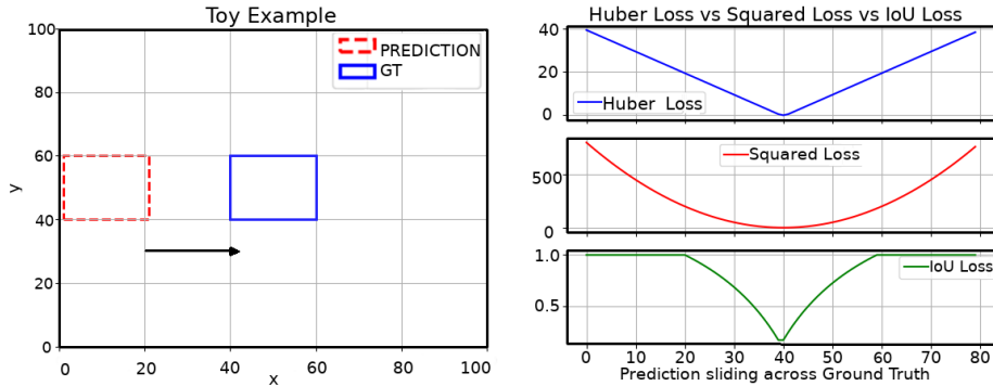
Fig. 1. The left figure mimicks the behaviour of a model predicting incrementally correct bounding boxes. The prediction is ‘slid’ over the ground-truth to examine the effect on the different losses. The figure on the right shows the behavior of the losses.
